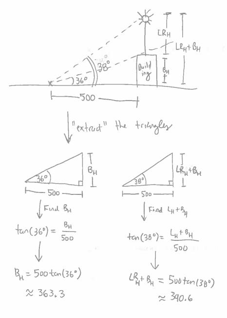
To find the height of the lightning rod - labeled LRH - we need to subtract the height of the building - labelled BH - from the total height of both the building and the lightning rod - labeled LRH+BH:
