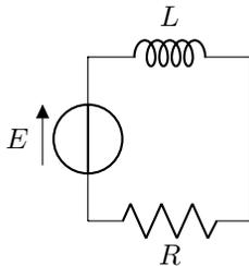
In a series circuit containing only a resistor ( $R$ , measured in ohms), an inductor ( $L$ , measured in henries which are ohm  $\cdot$  sec), and a current at
